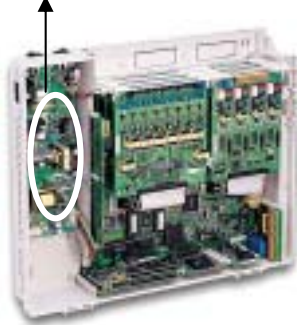
Figure 3. D1PWUA (POWER UNIT)
